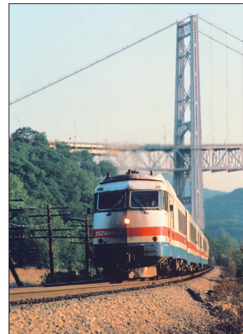
Amtrak Turboliner on the east shore of the Hudson River enroute from New York City to Albany, N.Y., after passing under Bear Mountain Bridge. Turboliners, with a top speed of 160 mph, were operated in partnership with the State of New York from 1974 to 2004.
